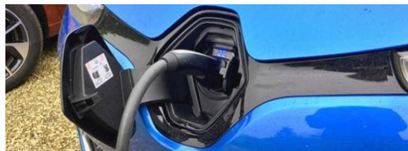
**Rapid** charging units (43, 50, or 120kW) can provide an 80% charge in around 30 minutes;
